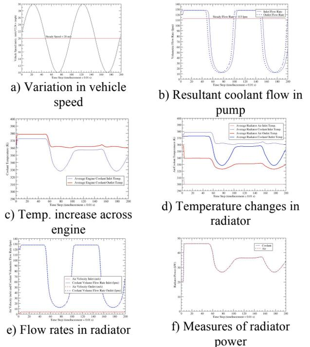
Figure 6: Ford Engine Cooling Loop Response to 50% Speed Perturbation
