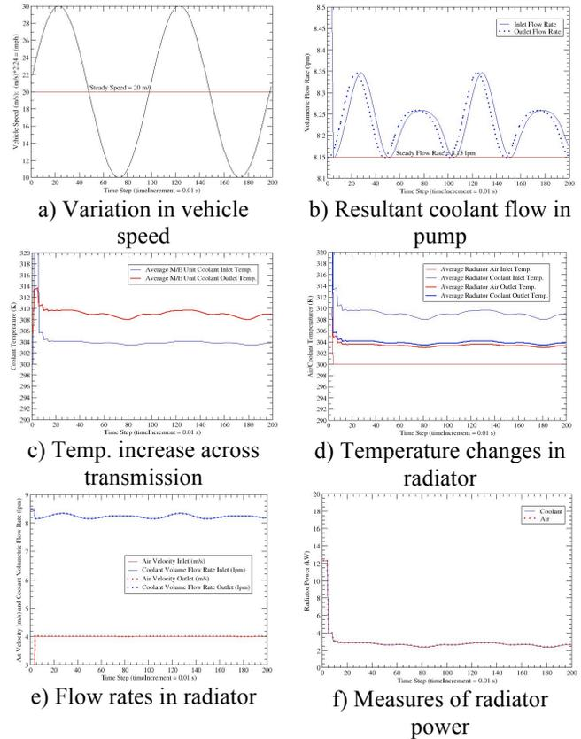
Figure 8: Ford Transmission Cooling Loop Response to 50% Speed Perturbation
