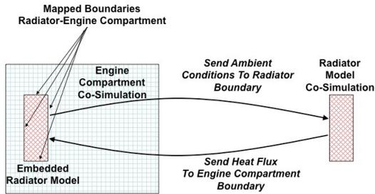
Figure 4: Data Exchange Between Reduced Models and the CFD Domain
