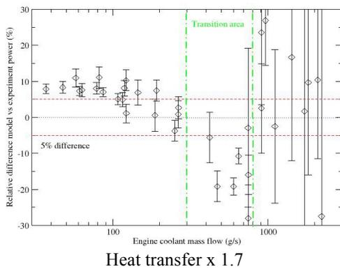
**Figure 14:** Comparison model/experiment data for engine coolant power for heat transfer factor=1.7
