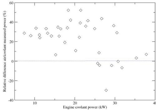
**Figure 13:** Relative differences between measured air and engine coolant powers
