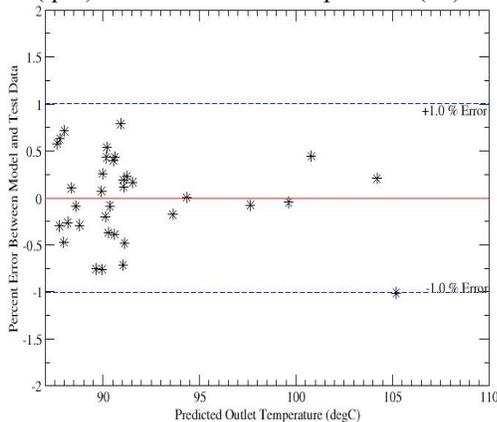
**Figure 23:** ANN-Engine model prediction of outlet temperature (°C)
