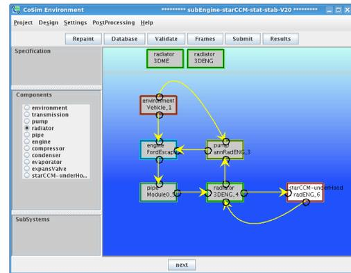
Figure 5: Modeling the Engine Cooling Loop
