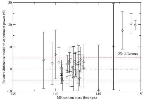
**Figure 16:** Comparison model/experiment data for transaxle coolant power, heat transfer factor= 2.6
