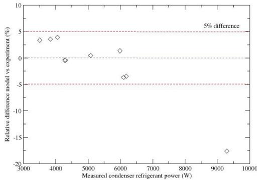
**Figure 22:** Comparison model/experiment for condenser refrigerant power; heat transfer factor = 0.8
