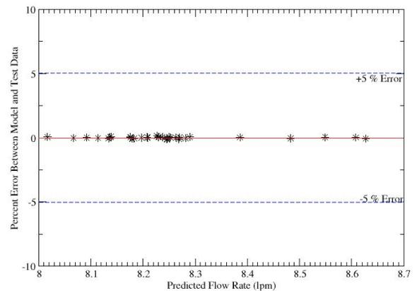
**Figure 25:** ANN-Pump model prediction of transaxle coolant flow rate (lpm)
