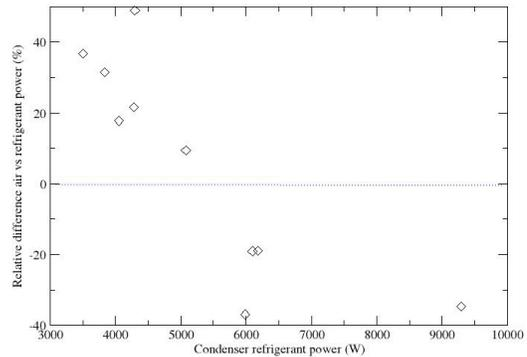
**Figure 21:** Comparison air/refrigerant measured powers (condenser, pruned valid data)
