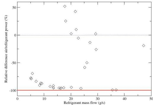
**Figure 17:** Comparison air/refrigerant measured powers (evaporator complete raw data)
