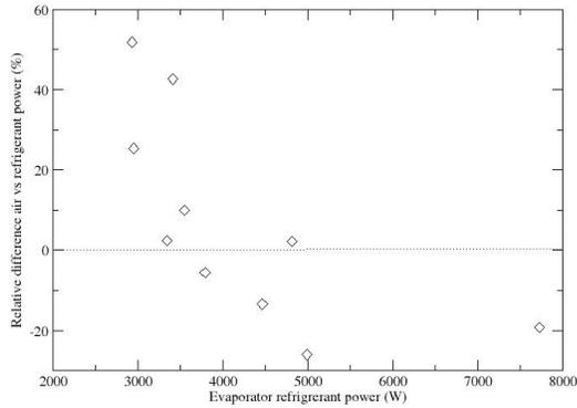
**Figure 18:** Comparison air/refrigerant measured powers (evaporator, pruned valid data)
