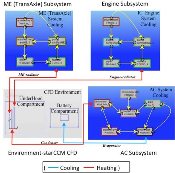
**Figure 11:** Schematic of the complete system
