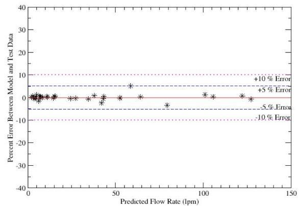
**Figure 24:** ANN-Pump model prediction of engine coolant flow rate (lpm)
