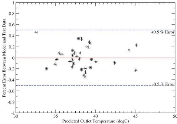
**Figure 26:** ANN-M/E Unit model prediction of outlet temperature (°C)
