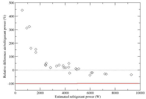
**Figure 20:** Comparison air/refrigerant measured powers (condenser, complete raw data)
